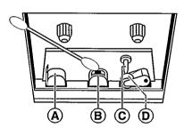
Use a cotton swab slightly moistened with cleaning fluid or alcohol.
